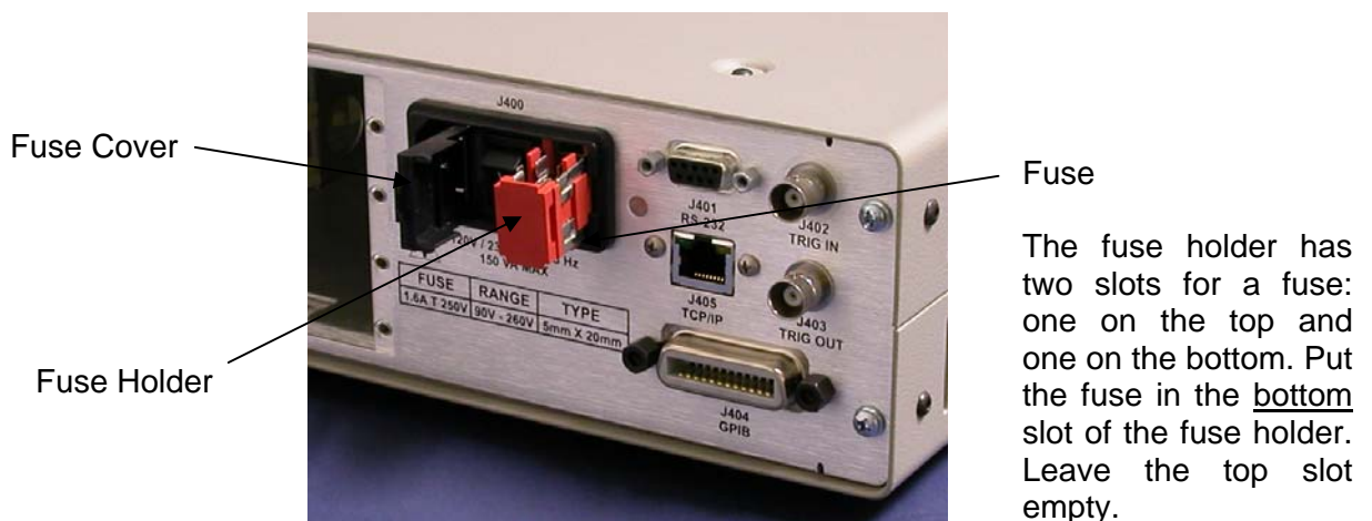
Figure 2-1, Changing Fuse for Main AC Power
