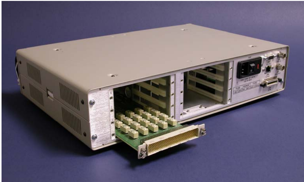
Figure 2-2, Inserting a Plug-In
